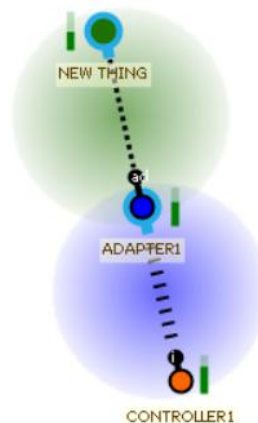
Figure 7 One Device (ADAPTER1) with an Established Connection as Peripheral (dotted line) and Concurrently Advertising (hashed line)
